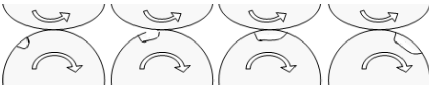
Figure 6.5: Flaking progression at a surface defect on the coating during slip-rolling
