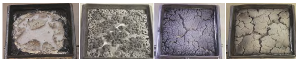
Fig 3.2.5. (a) HRRs and (b) the corresponding fire residue morphologies of EP and EP composites with different MMTs obtained in cone calorimeter under an external heat flux of 50 kW m -2
