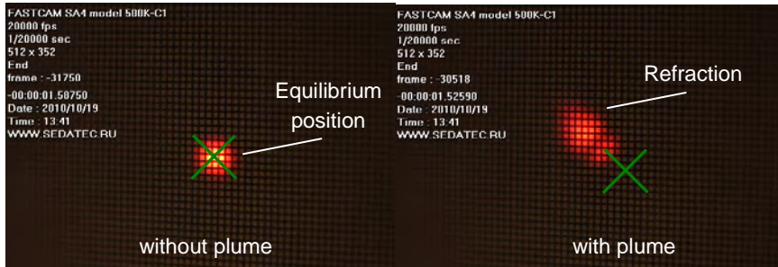
Fig. 3.2. Deviation of the probe beam spot position on the target surface due to the thermal refraction in the welding plume
