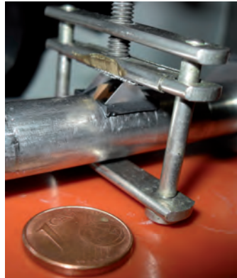
Figure 3.4: Image of a Au/TiO 2 coated prism installed on a pipe
