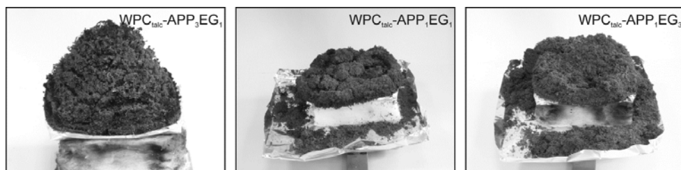
Figure 5.14: Residue after cone calorimeter measurement for WPC_{\text{talC}}\text{-APP}_3\text{EG}_1 , WPC_{\text{talC}}\text{-APP}_1\text{EG}_1 and WPC_{\text{talC}}\text{-APP}_1\text{EG}_3 at an irradiation of 50 \text{ kWm}^{-2}
