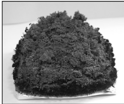
Figure 5.12: Residue after cone calorimeter measurement for WPC talc -EG 3 RP 1 measured under an irradiation of 50 kWm -2
