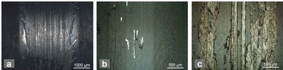
Figure 4-9: Defects of Fraunhofer IWS coatings at P_{0mean} = 1.5 \text{ GPa} in VP1 a) ta-C V5, b) ta-C V6 and c) a-C V7 (scale: a) 1000 \mu\text{m} , b) and c) 500 \mu\text{m} )
