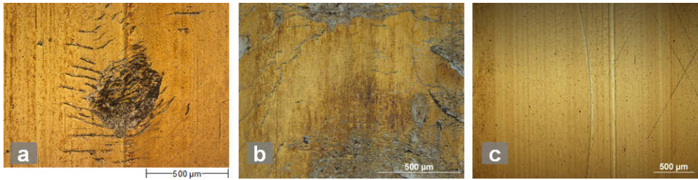
Figure 4-14: Sections of stressed and partial flaked Zr(C,N) wear tracks after a) 1.11 mio. cycles (V300), b) 4.98 mio. cycles (NC310YW) and c) 10 mio. cycles (CSS-42L) tested at P_{0mean} = 2.5 GPa and T = 120^{\circ}\text{C} (scale: 500 \mu\text{m} )
