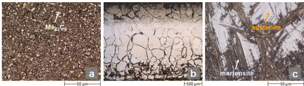
Figure 3-5: Microstructure of CSS-42L: a) \text{Me}_{23}\text{C}_6 carbides including martensitic case, b) transition zone below carburized case and c) core (etchant: \text{HNO}_3 and Marble, scale: a), c) 50 µm and b) 500 µm)
