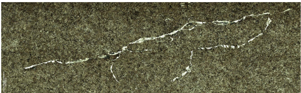
Figure 2-7: Optical image of white etching areas through inner ring of a wind turbine main shaft roller bearing in the cross section below stressed raceway
