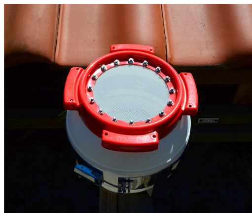
Fig. 2. The used low-cost bulk deposition sampler applied on a roof
