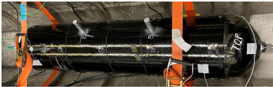
Fig. 4. Photograph of damage case setup. COPV with four masses glued onto the surface as artificial damage on different positions (D1-D4). The fourth damage (D4) is covered by the tension belt.
