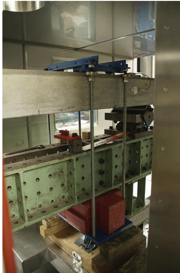
FIGURE 5: RC beam inside the climate chamber together with the substructure and moveable trolley with suspended weights.
