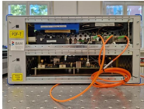
Fig. 2. Demonstrator - Digital I-OFDR device suitable for outdoor use in a robust and compact housing.
