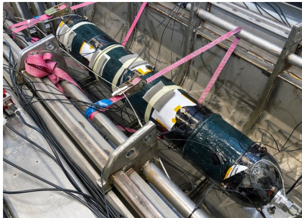
Fig. 1. Photograph of the experimental setup. The COPV is carried via tension belts inside the test rig (PN020) equipped with a hybrid sensor network consisting of AT, DFOS and GW sensors.
