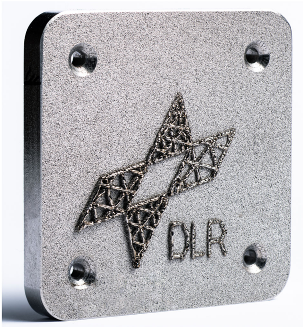
Fig. 7 Part built from eight layers from AMZ4 powder in microgravity. The part is completely welded to the platform, no detaching is observed. The surface of the build is mostly smooth and has a silvery shine.
