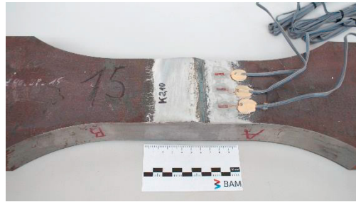
Fig. 2. Grinding of the weld toe transitions at specimen 2 and strain gauges positioning.
