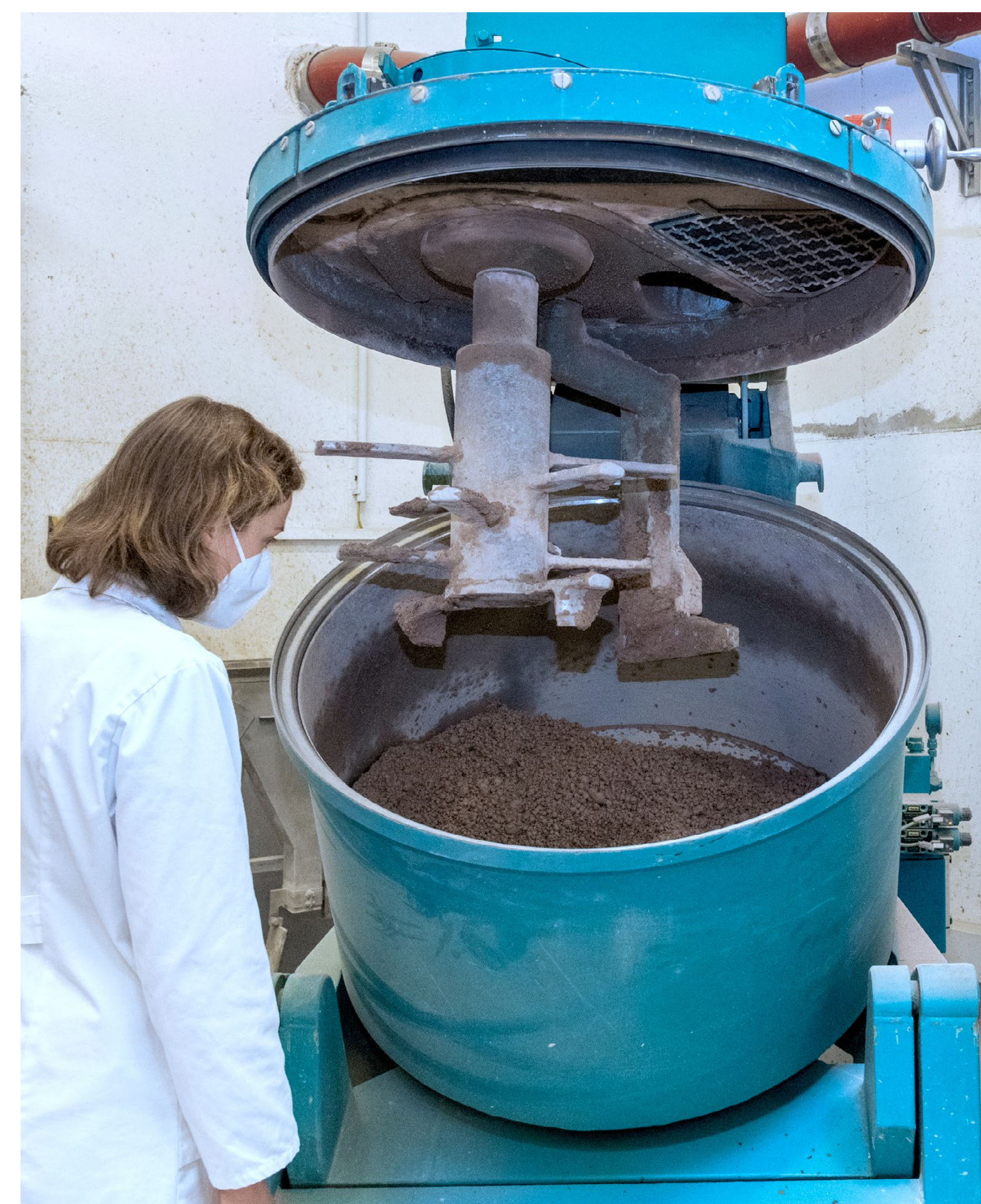
The granulate is processed into lightweight concrete in the intensive mixer.
