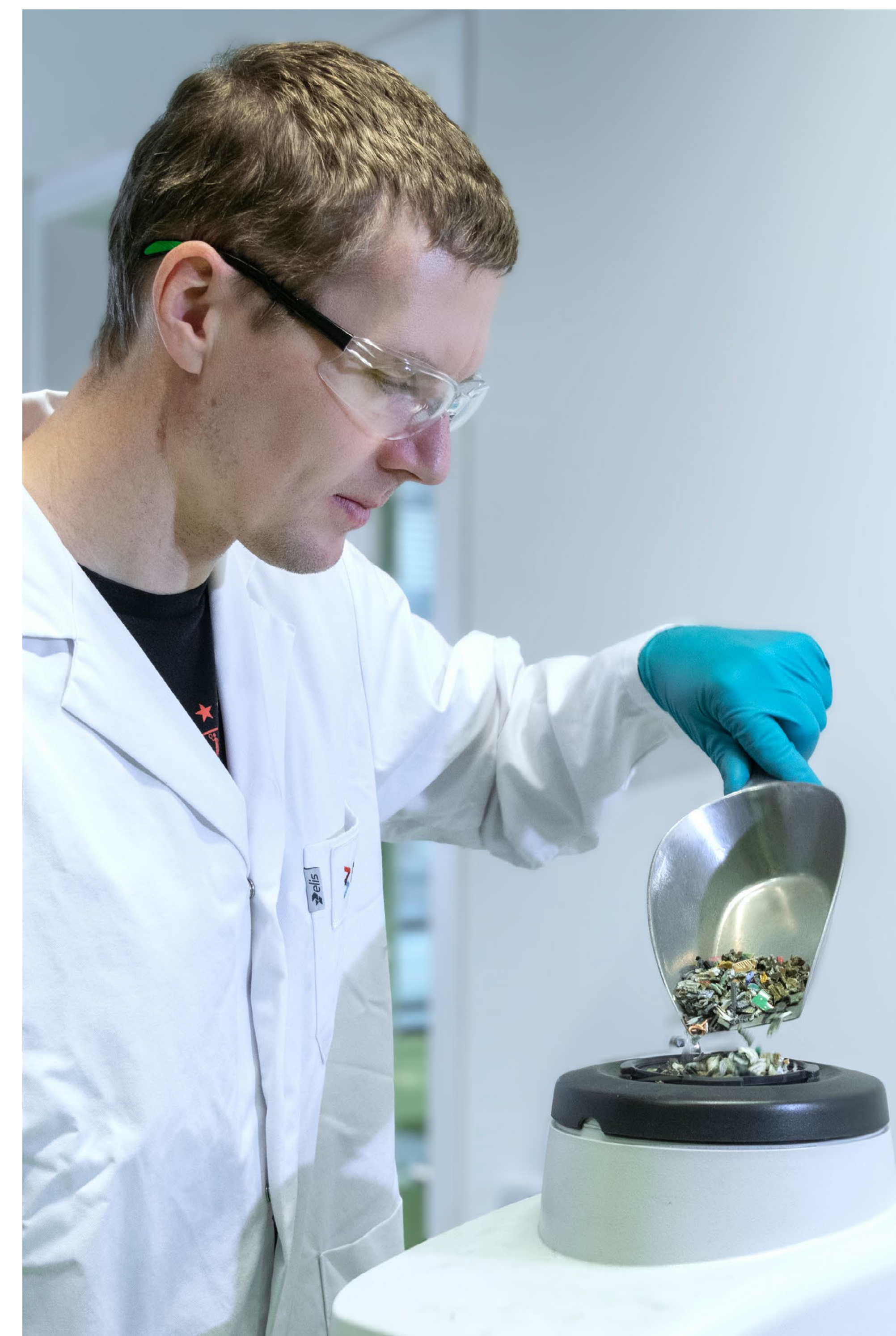
The coarsely crushed LED material is cooled and then finely ground.
