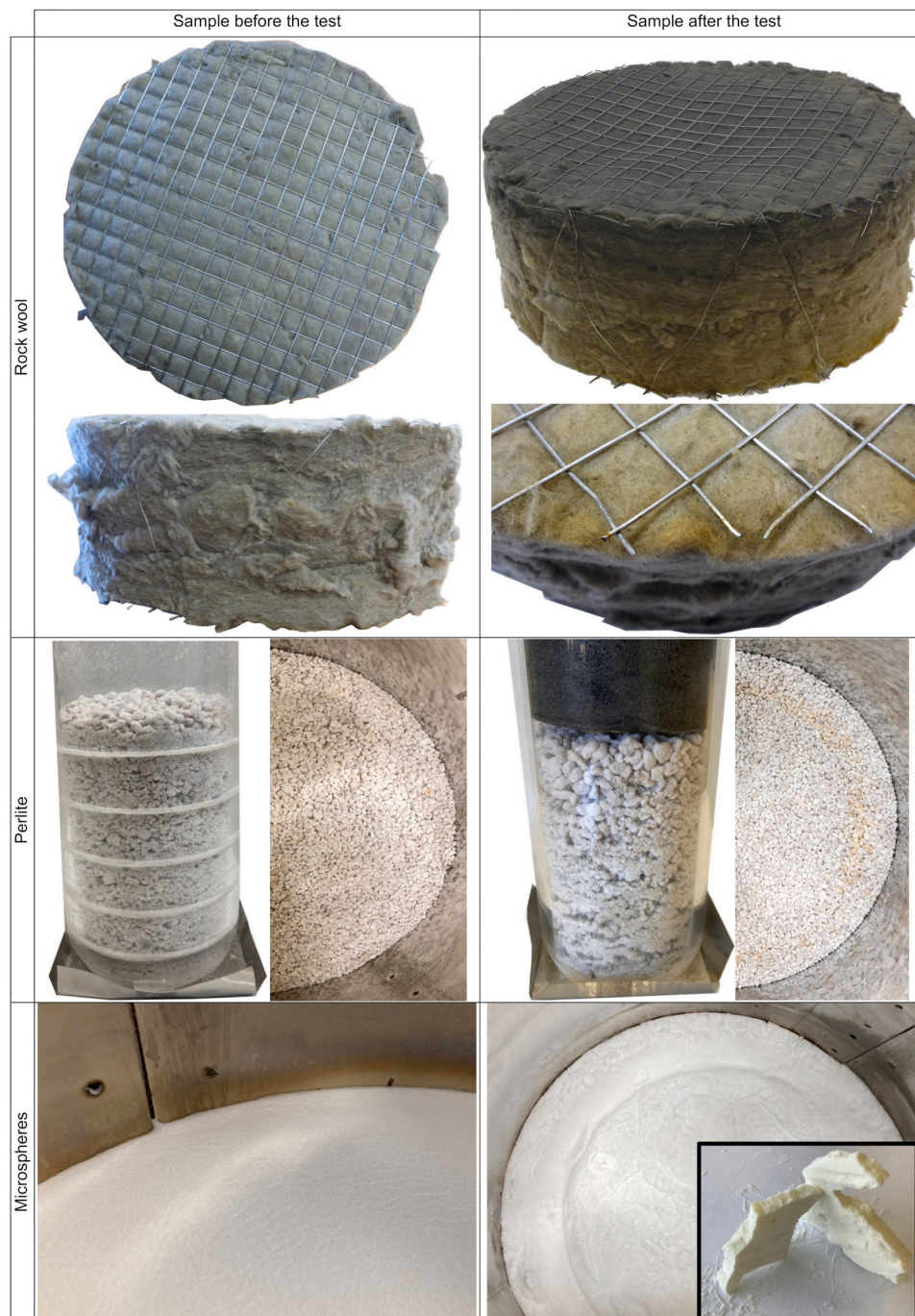
Fig. 6. Samples from the Rock wool, Perlite and Microspheres test before (left) and after thermal loading (right).
