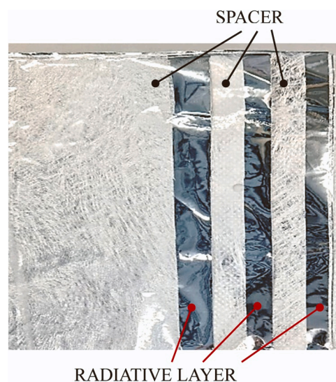
Fig. 2. An image of the tested MLI showing the alternated spacer and radiative layers.
