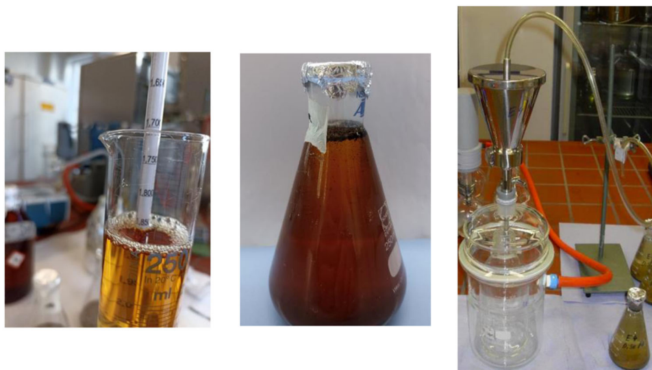
FIGURE 2 Determination of the density of the NaI solution (left); sediment sample in NaI solution (center); vacuum filtration system with suction device (right)
