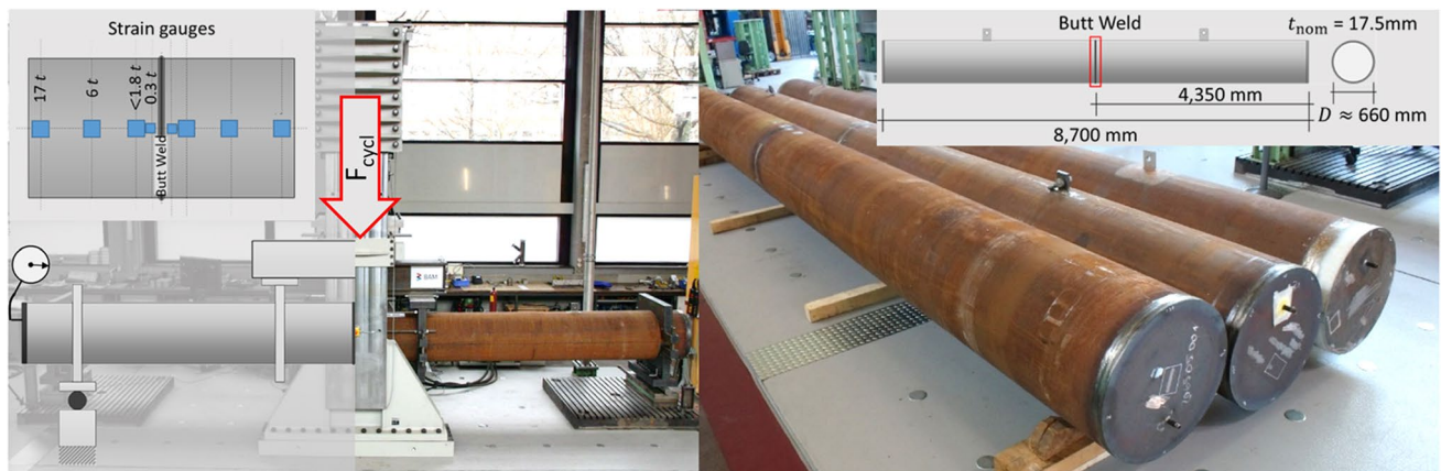
Fig. 10 Test rig at BAM Berlin for fatigue tests on tubes with butt-welded joints, geometry of the specimens, and position of strain gauges
