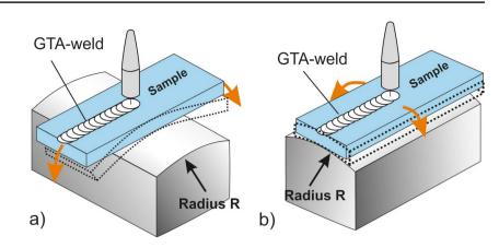
of Varestraint testing [4, 5]. There is not always an agreement in the literature about their respective influence on crack initiation, and the selection and evaluation of suitable parameters are still the subject of research [6]. Thomas et al. [7] provided a compilation of common parameter sets taken from technical standards, important publications, and selected recent studies.
