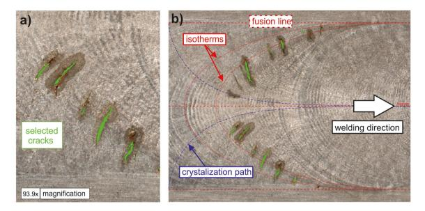
Fig. 6 Exemplary crack selection (a) and weld geometry selection (b); selected cracks in green; exemplary isotherms in red (solid line); exemplary crystallization paths in blue
