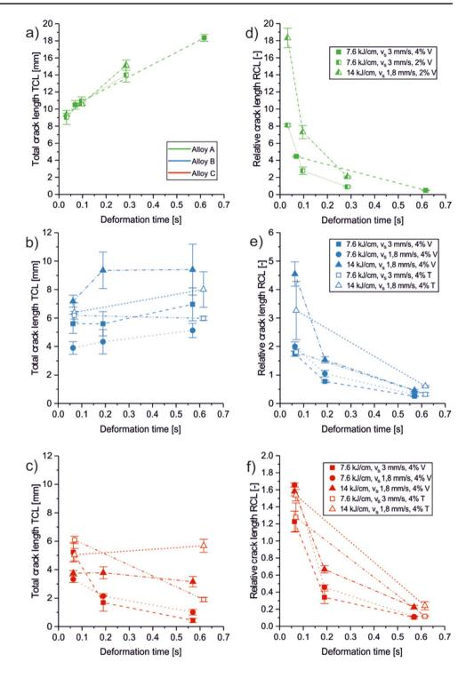
influenced by the MVT parameters. Nevertheless, RCL can also be used to compare the absolute solidification cracking susceptibility of several materials—if an identical MVT parameter range was applied. This is illustrated in the following.
