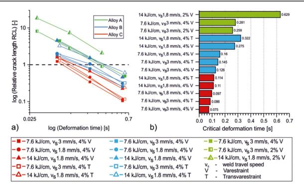
Fig. 8 Relative crack length RCL (log) as a function of the deformation time applied (a) and critical deformation time  $d_{def,1}$  calculated for all parameter sets (b)
