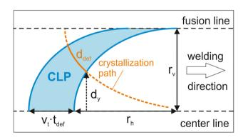
**Fig. 3** Deformation-induced crack length  $d_{def}$  along the crystallization path during deformation at the distance  $d_y$  from the weld centerline;  $v_t$ , weld travel speed;  $t_{def}$ , deformation time;  $r_h$ , horizontal weld radius;  $r_{v_r}$  vertical weld radius. The integral of all  $d_{def}$  is the crack length potential CLP
