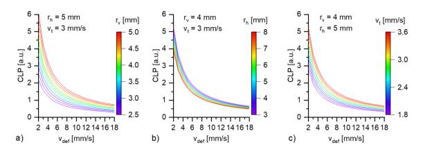
Fig. 5 Influence of different test parameters on the crack length potential CLP, plotted as a function of the deformation speed  $v_{def}$ . Vertical weld pool radius (**a**), horizontal weld pool radius (**b**), and weld travel speed (**c**)
