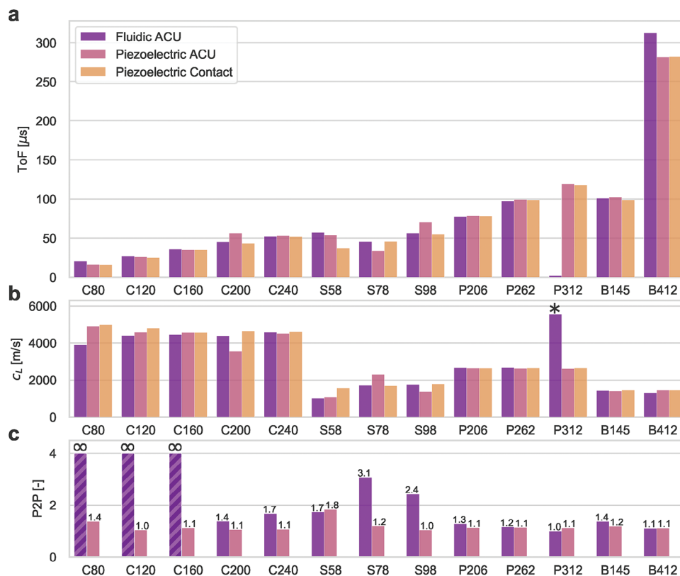
Figure 4. Measurement results of the fluidic transducer compared to the piezoelectric and contact transducer. The specimens are abbreviated using the initial letter of their material followed by their thickness in mm, e.g., C160 is the concrete specimen with a thickness of 160 mm. All specimens used in this study are tabulated in the experimental section. a) ToF. b) Longitudinal velocity c_L . The bar referring to the fluidic transducer results for specimen P312 (*) is cropped. The actual velocity is calculated to be 156000 \text{ ms}^{-1} . c) Peak-to-peak ratio (P2P) of the cross-correlation output. The \infty sign for the P2P of the fluidic transducer transmitting through the first three concrete specimens indicates that no second peak was found, so the P2P would approach infinity. Data from the contact transducer is not included as the P2P measure is applicable only to the ACU measurements.
