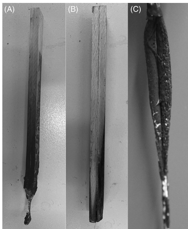
FIGURE 7 UL 94 vertical test of (A) polycarbonate 4.1 mm, (B) wood 8.1 mm, (C) ABS 2.1 mm.
