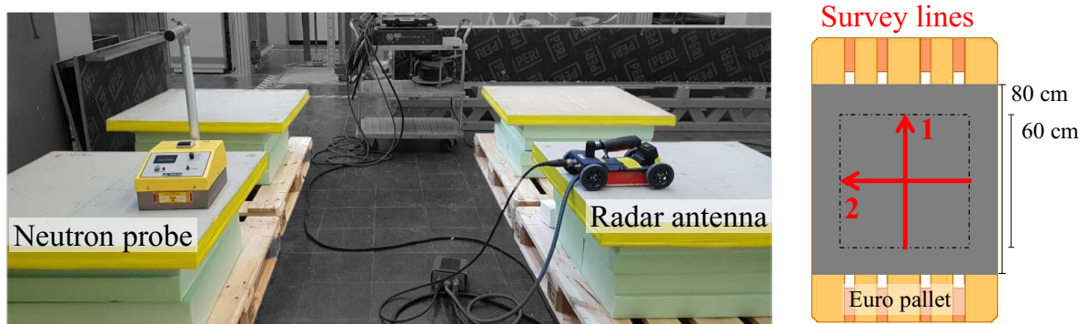
Figure 2.4: Measurement setup with neutrone probe and radar antenna on screed test specimens. The right graphic shows the perpendicular orientation of the two recorded GPR survey lines on a screed in top view
