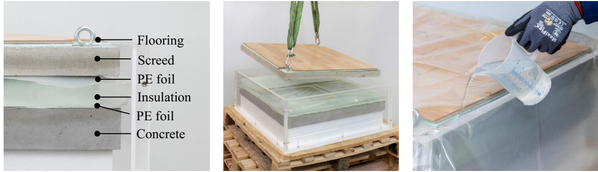
Figure C.1: Modular test specimen with screed, insulation, and concrete base layer (left, middle) and the simulation of an insulation damage by adding water to the setup (right).
