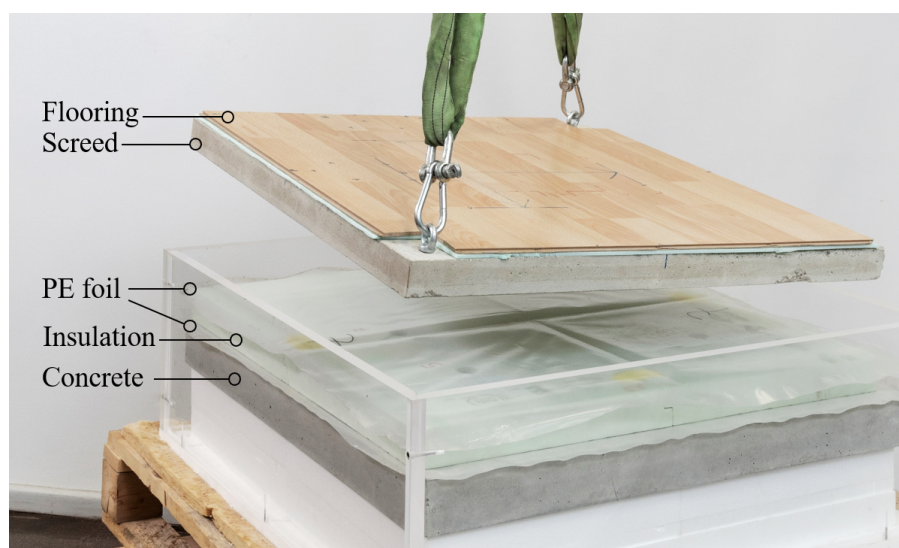
Figure B.3: Modular test specimen with screed, insulation, and concrete base layer.
