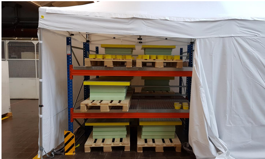
Figure 2.3: Storage of the samples in a climate controlled tent at 23 °C and 50 % RH.
