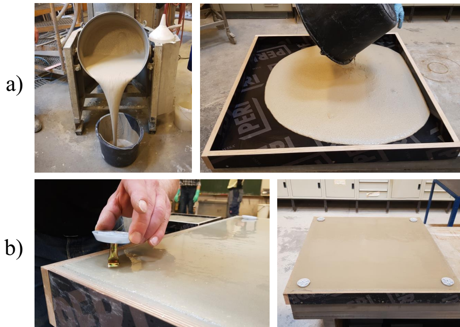
Figure 2.2: Casting of screed samples: a) Freshly mixed CA screed gets poured into its formwork. b) Embedding of threaded sleeves into each corner to enable handling with ring bolts.
