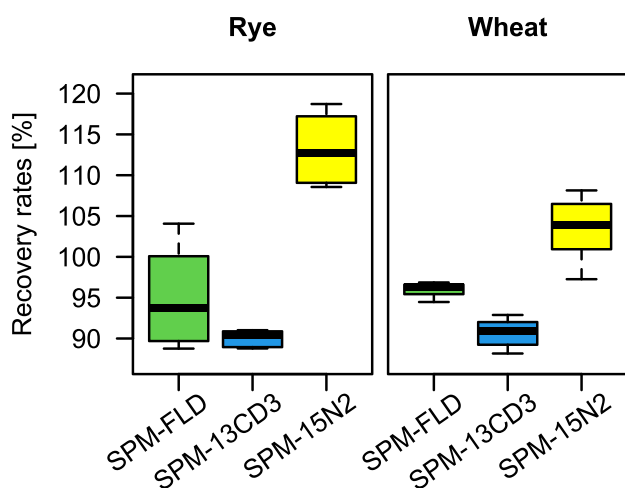
Fig. 5 Determined recoveries of the FLD-based sum parameter method (SPM-FLD) and the MS/MS-based SPMs employing either ^{13}\text{CD}_3 - (SPM-13CD3) or ^{15}\text{N}_2 -labelled (SPM-15N2) lysergic acid hydrazide as IS in rye or wheat flour. Matrices were doped with a mix solution containing equimolar amounts of each major ergot alkaloid and analyzed in fourfold replicates with double injection
