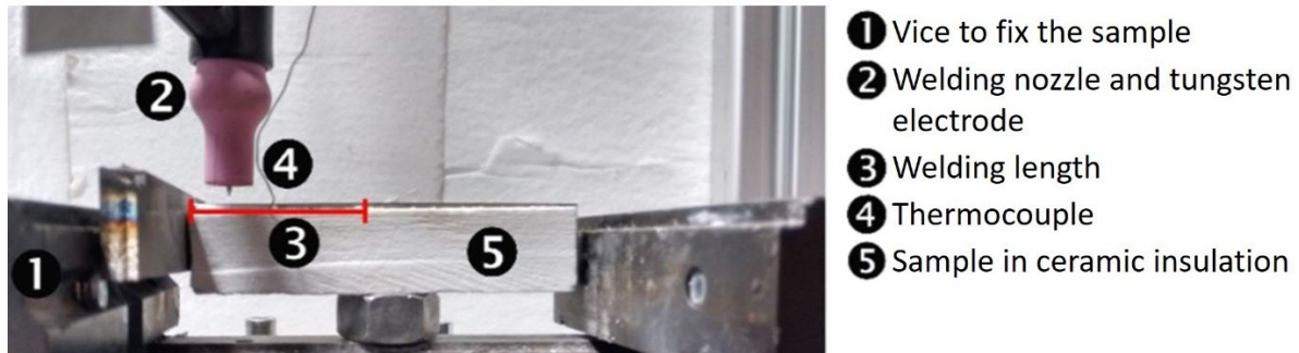
Figure 1: Photo of the welding set-up with the view in neutron flight direction [25]. A parallel clamping device fixes the sample. Alumina felt (white) around the sample reduces thermal losses allowing for longer exposure times. Welding takes place at the narrow side.
