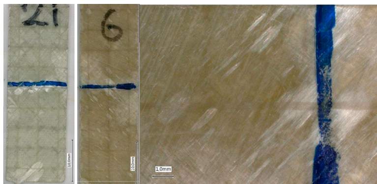
Fig. 7. Microscopy of GFRP specimens showing signs of delamination (left: dry configuration; right: wet aged configuration).
