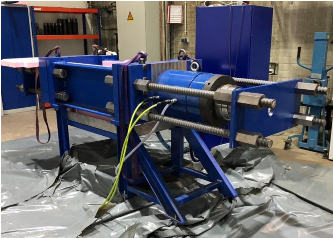
SAH-Figure 9: After completion, the newly built 3 MN stress corrosion cracking test rig at SAH.
