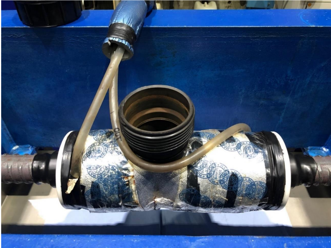
SAH-Figure 11: Conventional test vessel according to DIN EN ISO 15630-3:2020-02, incl. curing tube.
