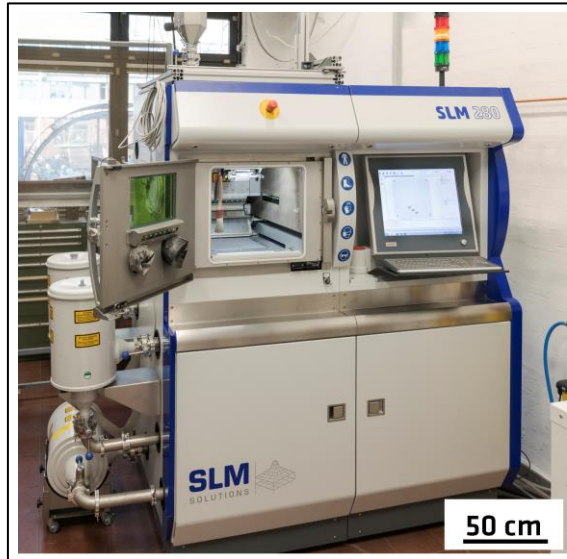
Figure 3.1: The PBF-LB/M machine SLM Solutions 280HL (SLM Solutions Group AG, Lübeck, Germany) used for the manufacturing of the 316L specimens.
