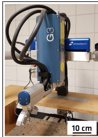
Figure 3.11: Xstress G3 mobile diffractometer (StressTech Oy, Vaajakoski, Finland).
