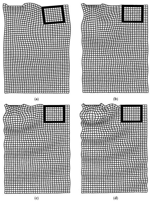
Figure 10. The vibration mode of a concrete block at (a) 20, (b) 40, (c) 60, and (d) 80 Hz.
