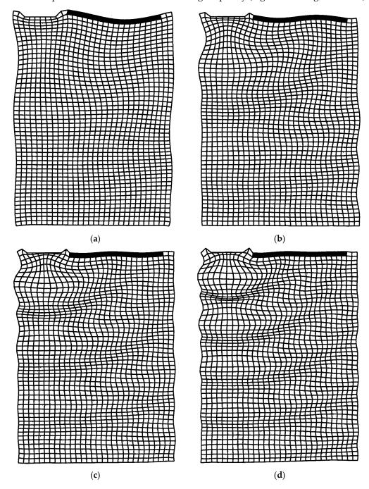
Figure 9. The vibration mode of a concrete plate at (a) 20, (b) 40, (c) 60, and (d) 80 Hz.
