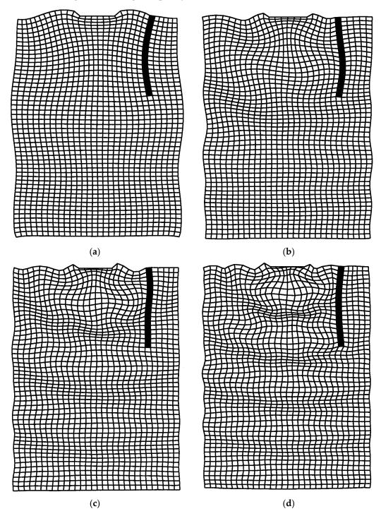
Figure 8. The vibration mode of a concrete wall at (a) 20, (b) 40, (c) 60, and (d) 80 Hz.
