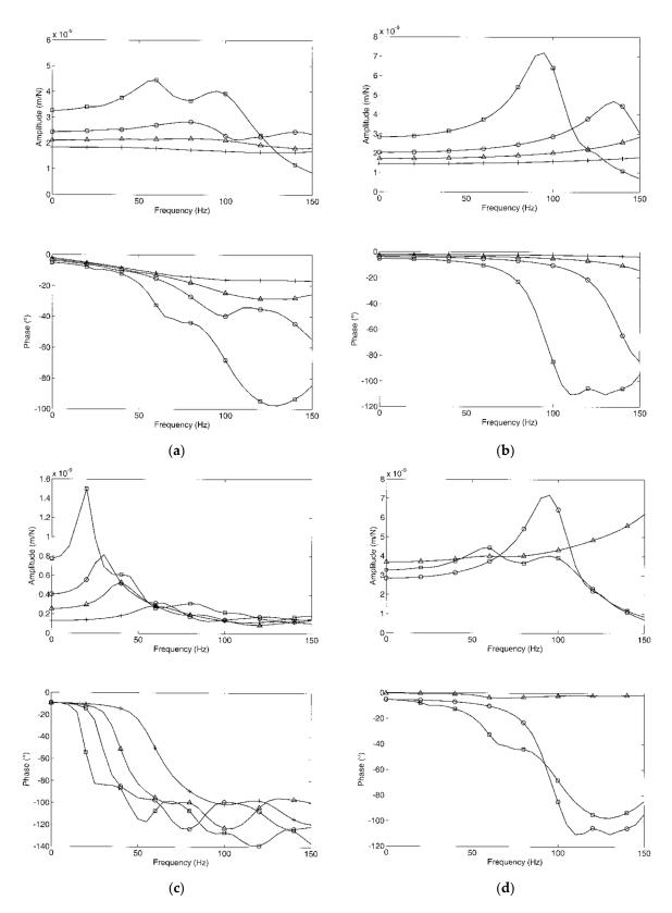
**Figure A1.** Compliances of different tracks: (a) ballasted track on the soil, (b) ballasted track on the bridge, (c) slab track on a sub-soil layer (compliance of the plate) variation in the ballast or subsoil  $v_S = \Box 100, \odot 150, \bigtriangleup 200, +300 \text{ m/s in } (\mathbf{a-c})$ . Comparison of the rail compliances (d) for the ballasted track on the soil  $\Box$ , the ballasted track on the bridge  $\bigcirc$ , and the slab track  $\bigtriangleup$ .
