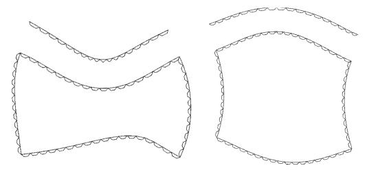
**Figure 2.** Boundary-element model of a tunnel, the soil is represented by the full-space solution and the stress-free surface above the tunnel has to be modelled.
