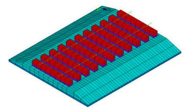
**Figure 3.** Finite-element model of a railway track including 2 rails, 11 sleepers with 22 rail pads, under sleeper pads, ballast, under-ballast mat, the soil is represented by the boundary-element method and the Greens' functions of the half-space.
