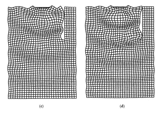
Figure 6. The vibration mode of an open trench at (a) 20, (b) 40, (c) 60, and (d) 80 Hz.
