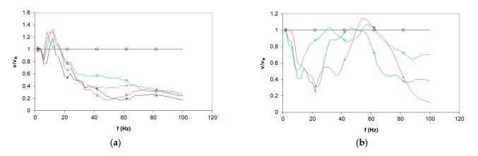
**Figure 12.** The frequency-dependent reduction effect of (**a**) cuts with different inclinations of  $\Box$  0 (reference),  $\bigcirc$  1:2,  $\triangle$  1:1, + 2:1,  $\times \infty$  (vertical) and (**b**) embankments with different inclinations of  $\Box$  0 (reference),  $\bigcirc$  1:2,  $\triangle$  1:1, and + 2:1, compared to the reference case of a surface line.
