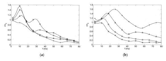
**Figure 14.** The frequency-dependent reduction effect of the tunnel excitation compared with a line load: (a) with variation in the thickness of the tunnel wall  $\Box$  0.3,  $\bigcirc$  0.5,  $\triangle$  0.7, + 1.0 m; (b) and variation in the wave velocity of the soil  $v_S = \Box$  150,  $\bigcirc$  200,  $\triangle$  300, + 500 m/s.
