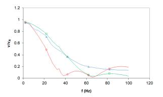
**Figure 5.** The soil amplitudes *v* averaged at 20 to 30 m distance for  $\Box$  a strip load of *b* = 3 m,  $\bigcirc$  a strip load of *b* = 5 m, and  $\triangle$  a load on a rigid strip foundation (*b* = 3 m), compared to the averaged reference amplitudes *v*<sub>R</sub> of a line load (the frequency-dependent reduction effect *v*/*v*<sub>R</sub>).
