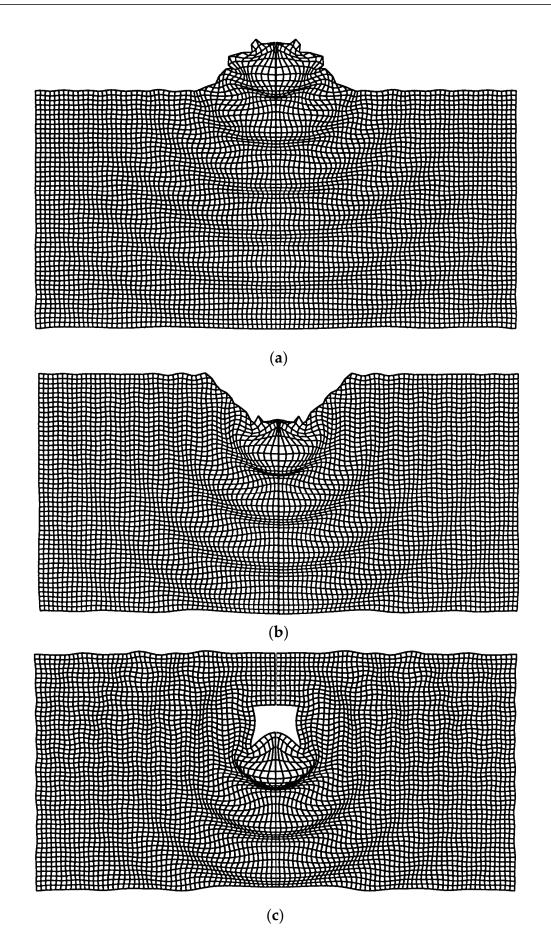
Figure 11. The vibration mode at 80 Hz of (a) a dam, (b) a cut, and (c) a tunnel.
