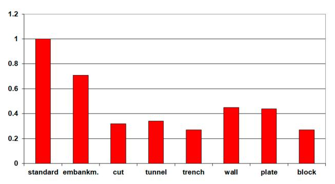
**Figure 15.** The reduction effect of different railway lines and different obstacles for frequencies between 40 and 80 Hz (average).
