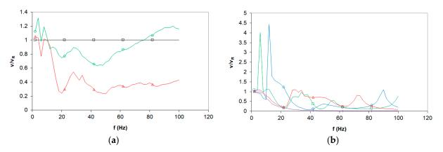
**Figure 13.** The frequency-dependent reduction and amplification effect (**a**) of tunnels at depths of  $\triangle$  10 m and  $\bigcirc$  5 m (concrete cut); (**b**) of bridges with span lengths  $\square$  15,  $\bigcirc$  10,  $\triangle$  5 m, and + a concrete bridge pier of 5 m × 5 m.
