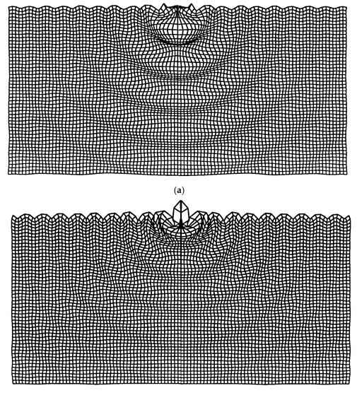
**Figure 4.** The vibration mode at 80 Hz for (**a**) a rigid strip foundation (representing the track) and (**b**) a concentrated line load.
