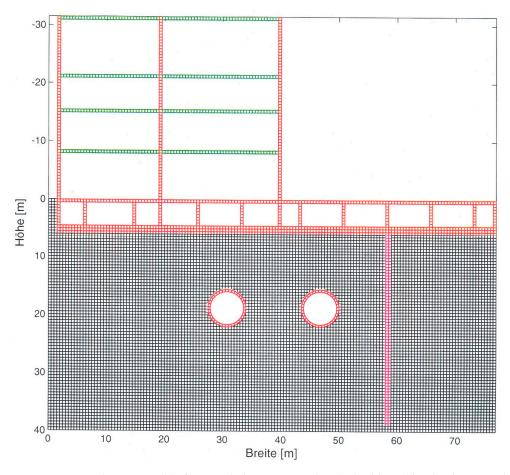
**Figure 1.** Finite-element model of a tunnel, the interior soil and a building; (the thin layers at the left and right boundary and the viscous dampers at the bottom are not shown).
