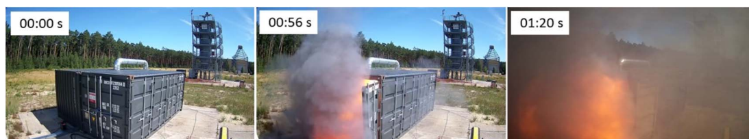
Fig. 13 Test #09, subsequent gas explosion due TR and pressure release of the experimental room.
