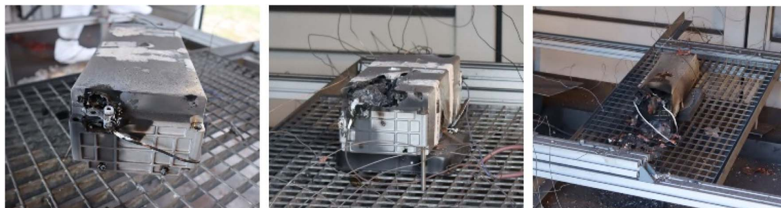
Fig. 9 Damaged tested modules from: test #07 (left), test #08 (middle), and test #09 (right).
