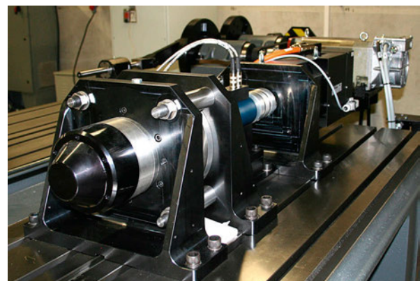
Figure 2.1: Test Bench for Tribological Characterization of Seals © TEKNIKER
