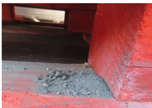
FIGURE 6 Release of toxic substance (UN 3288) from the closure of a 13H3 woven plastics FIBC (Police North Rhine-Westphalia Münster).
