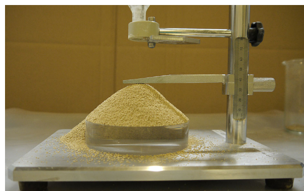
FIGURE 10 Method according to ISO 4324—Measurement of the height of powder cone using the slewable measuring bar (Biathlon 4D).
