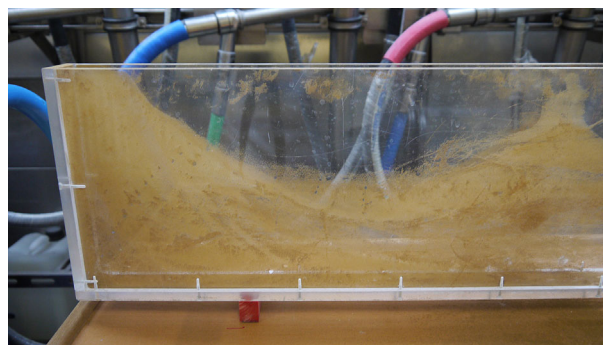
FIGURE 22 'Plate method' (plexiglass)—Apparatus with dust deposits after testing cantus.
