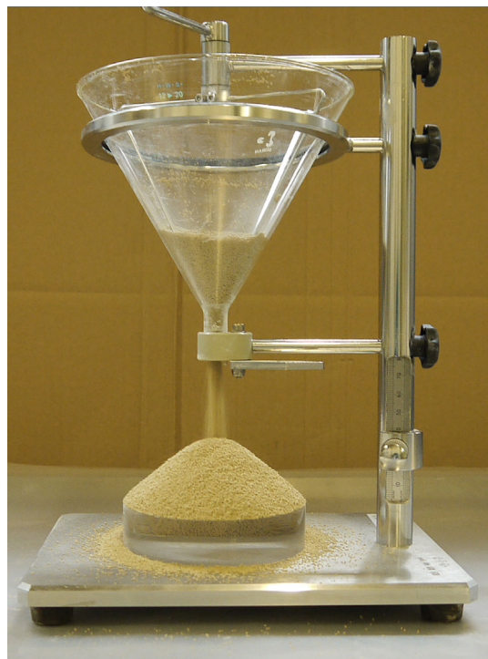
FIGURE 9 Method according to ISO 4324—Biathlon 4D during the discharge process from the funnel.
