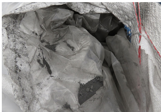
FIGURE 5 Release of toxic substance (UN 3288) from the closure of a 13H3 woven plastics FIBC (Police North Rhine-Westphalia Münster).
