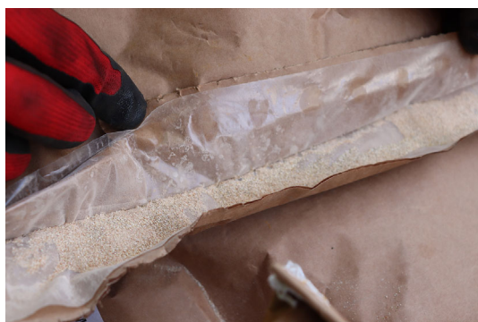
FIGURE 3 Release of an environmentally hazardous substance (UN 3077) from the stitched join of a 5M2 paper bag (Police North Rhine-Westphalia Münster).
