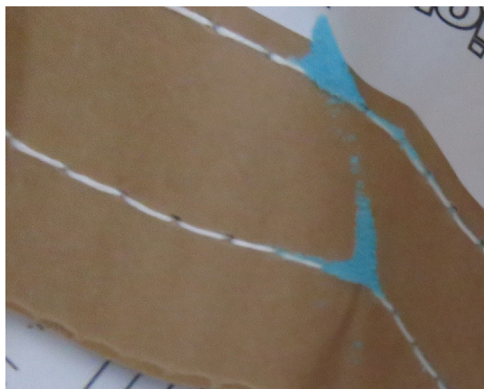
FIGURE 2 Release of an environmentally hazardous substance (UN 3077) from the stitched join of a 5M2 paper bag (Police North Rhine-Westphalia Münster).
