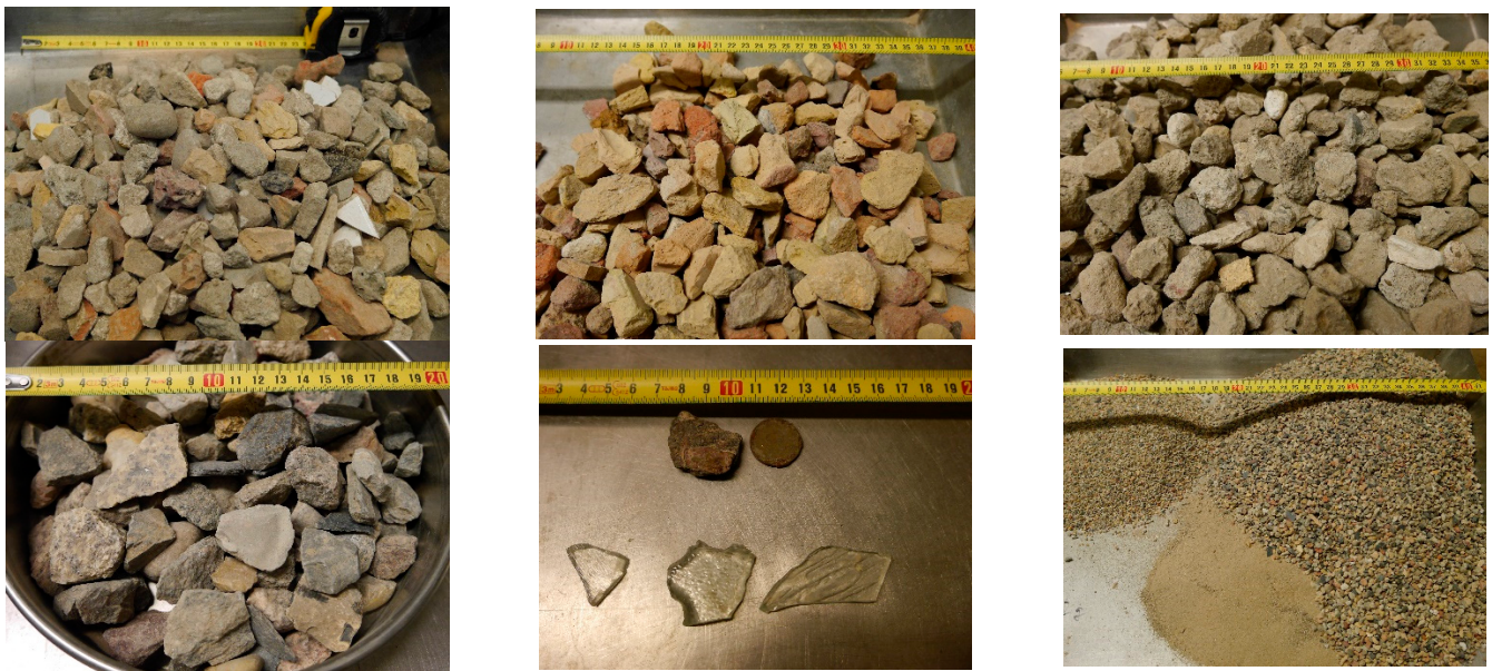
Figure 3. Photos of the individual material groups and screen fractions (from top left to bottom right: >16 m unsorted, >16 mm bricks (25.8%), >16 mm mortar (50.6%), >16 mm stones (14.2%), >16 mm glass and metals (0.4%), and sieving fractions <0.63, <2 and <4 mm together). Material group “ceramics” (9%) not illustrated. (Photographs by F.-G.S.).
