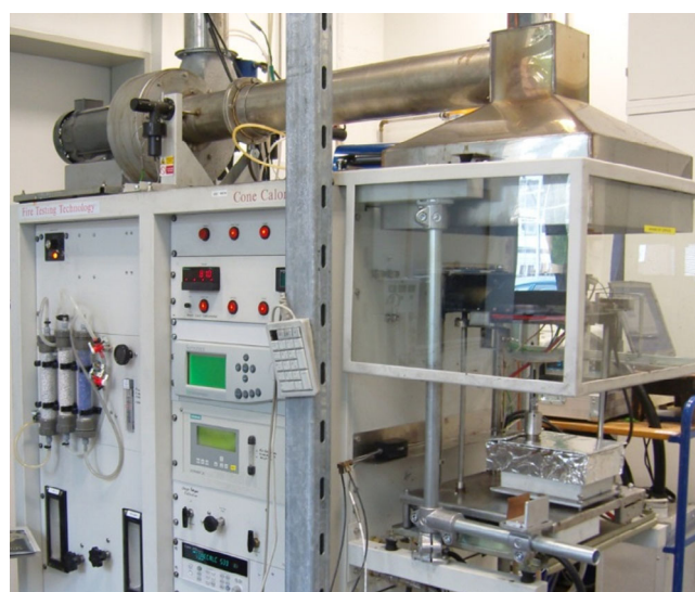
FIGURE 4 Cone calorimeter set-up at the BAM Lab.
