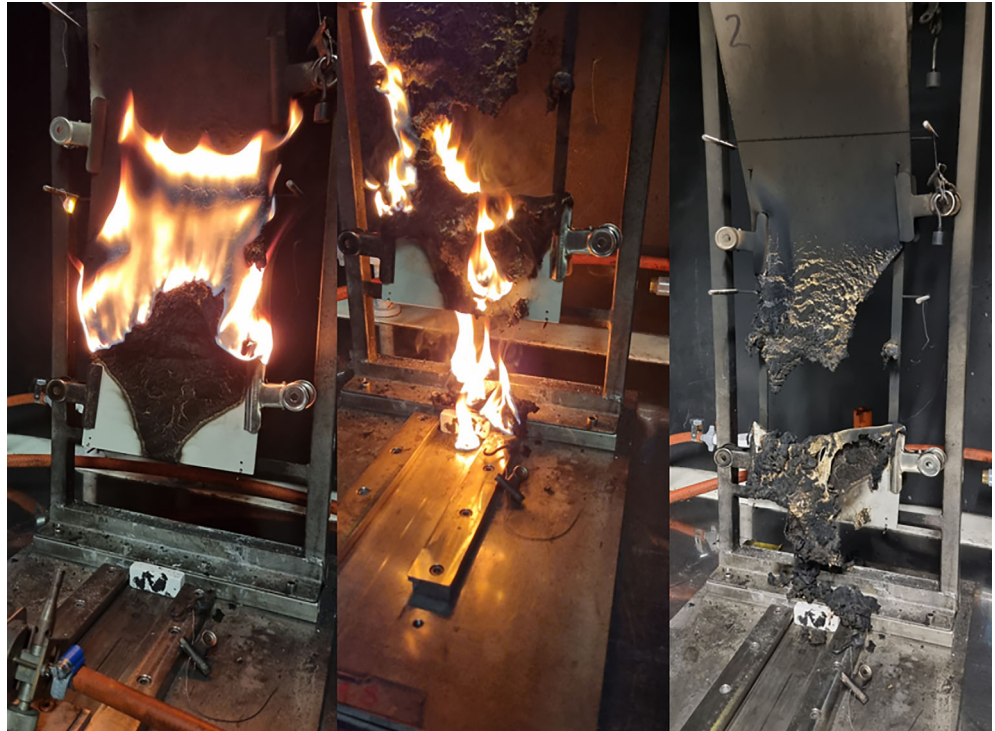
FIGURE 4 Fire testing of a PC/ABS material according to R 118, Annex 8.
