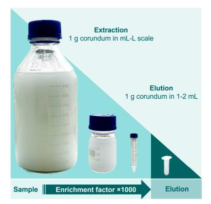
**Figure 8.** Reduction of a sample volume between 100 and 1000 mL resulting in a final elution volume down to 1 mL (schematic representation).
