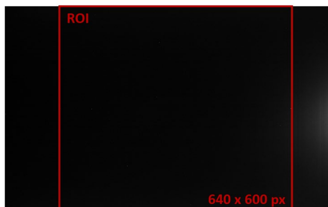
Figure S11. Images of the CMOS with 2x2 pixel binning resulting in an image size of 900x600 px. Highlighted region of interest (ROI, 640x600 px; ROI file for script.py can be found in the supplementary materials named: roi_region_x_y.txt, as well as the hot pixels file: hotpixels_960_600.txt for the biosensor measurements with an exposure time of 15 sec.
