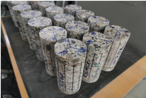
Fig. 1. Drilled cores prepared for testing.
