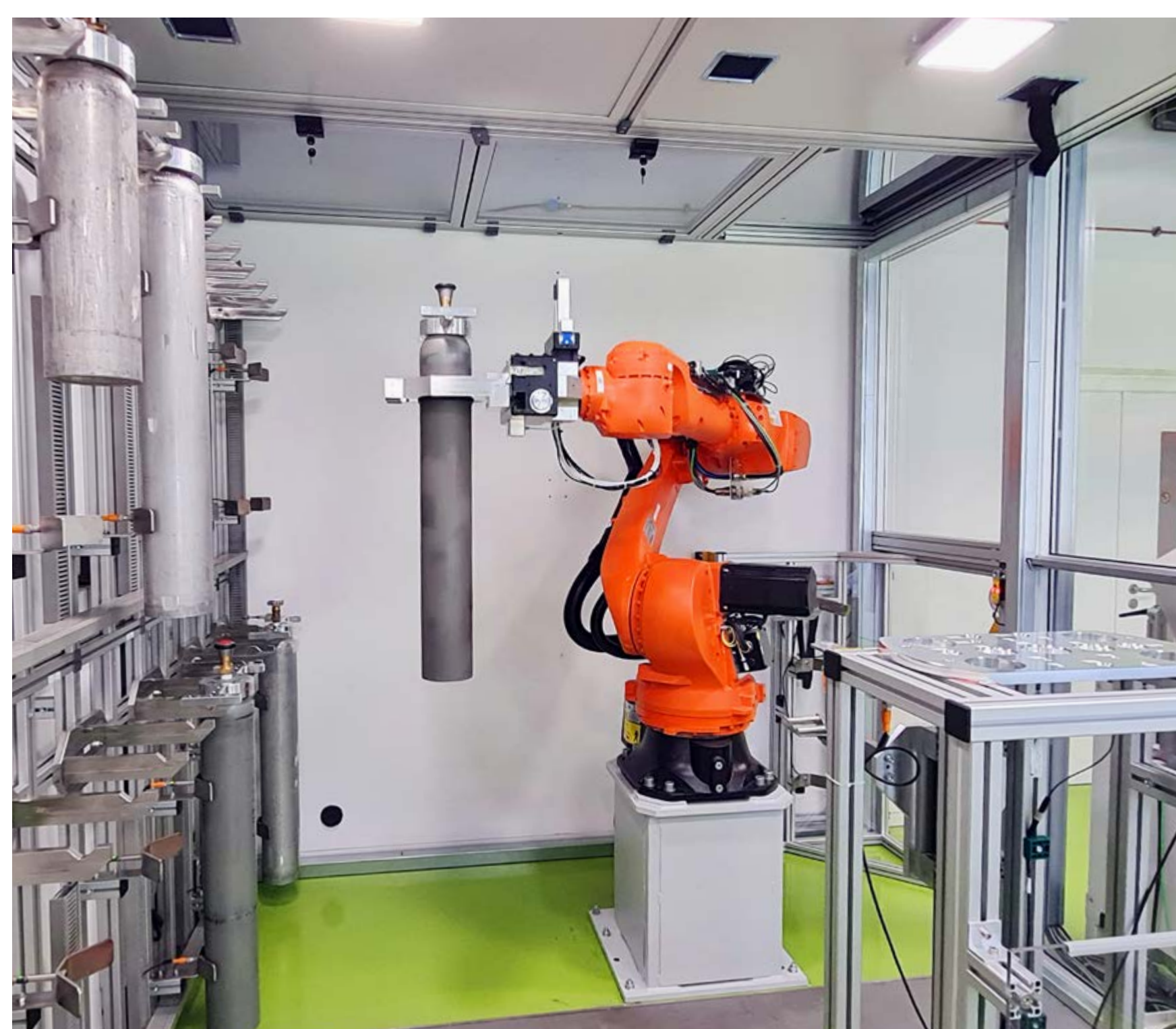
With the aid of a weighing robot, BAM produces highly accurate calibration gases.
