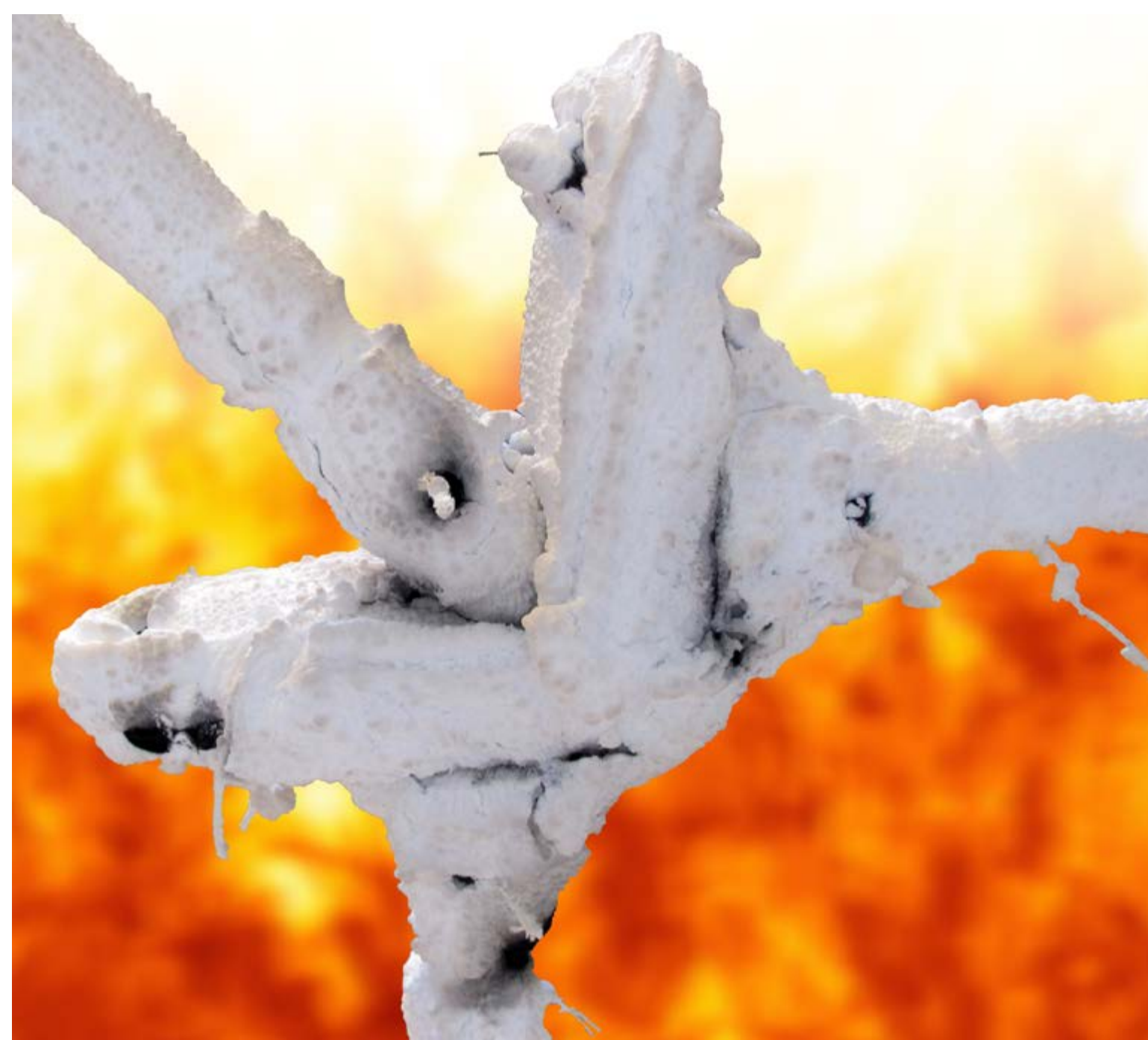
Reactive fire protection systems create a thermal protective char that delays the heating of the steel
