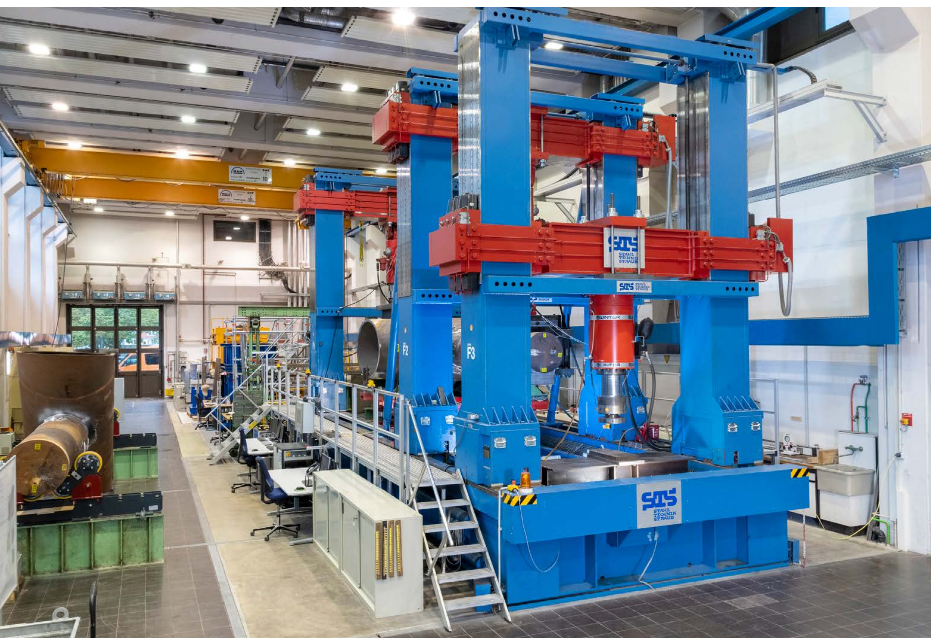
In the large-scale test rig of the Competence Centre, steel components are undergoing stress tests with different loads.
