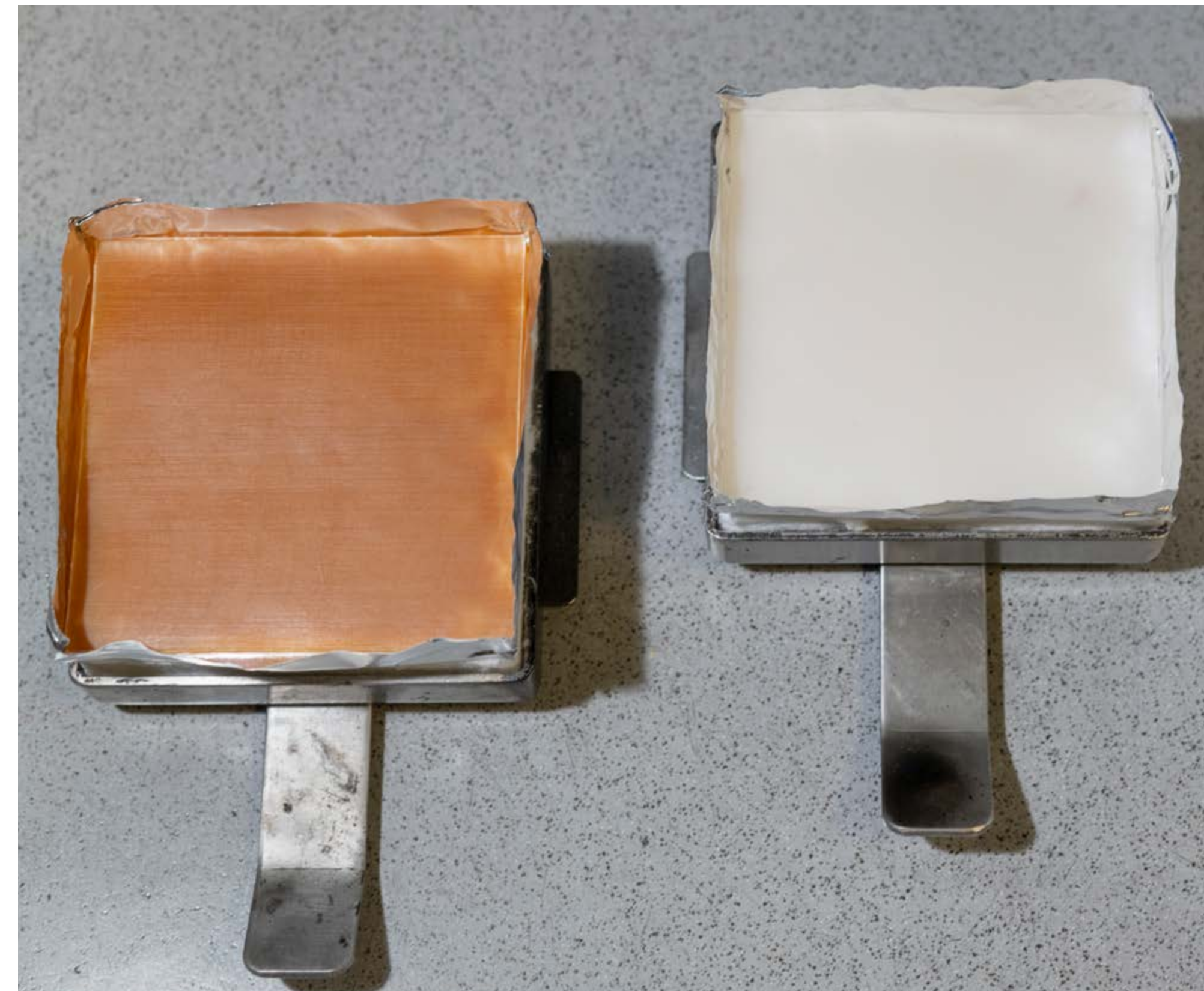
Flame protection made of leather fibres (l.) develops a charred surface when it burns (r.), which acts like a heat shield
