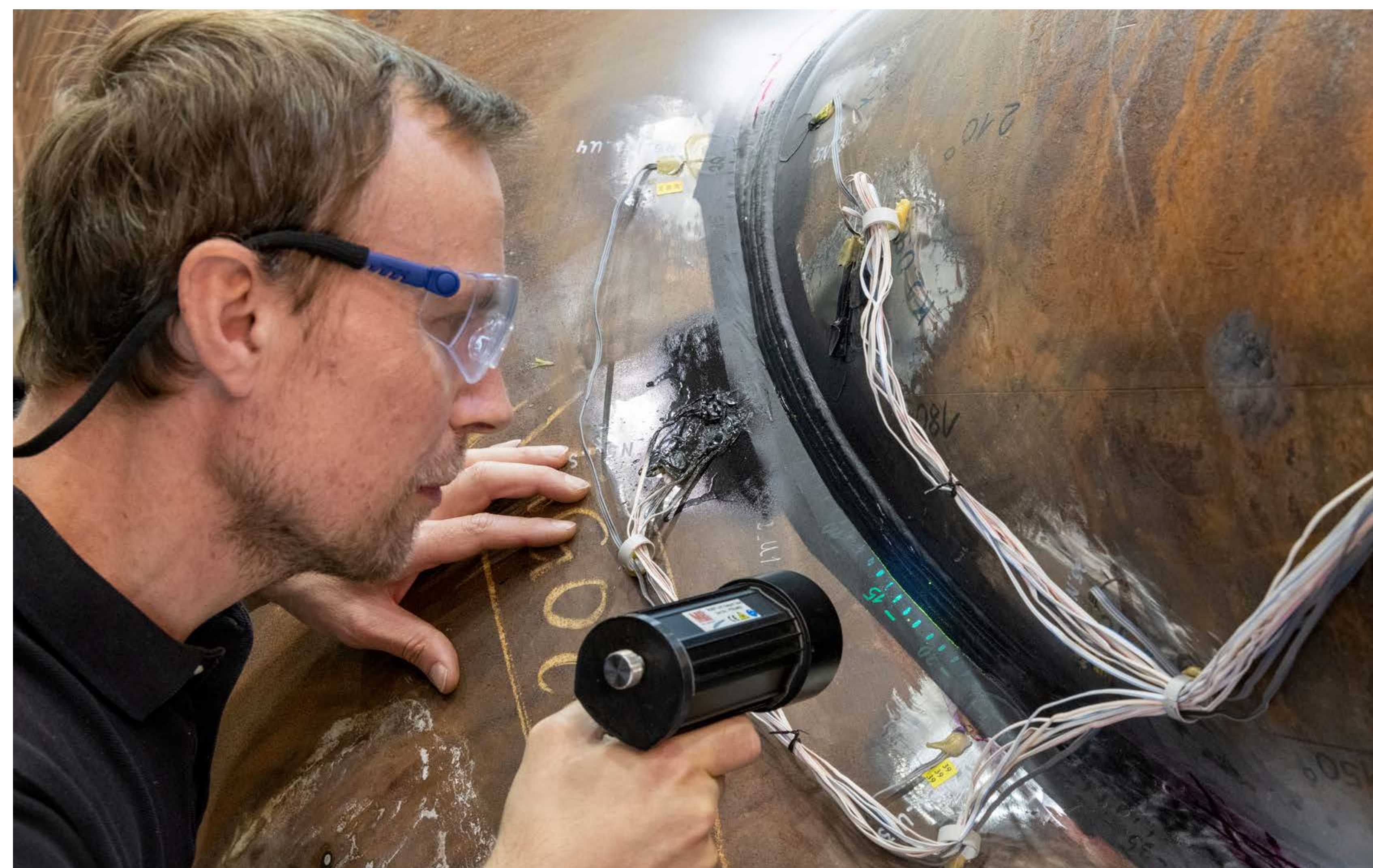
Fluorescence can be used to examine welding seams on the support structures of wind turbines for cracks.
