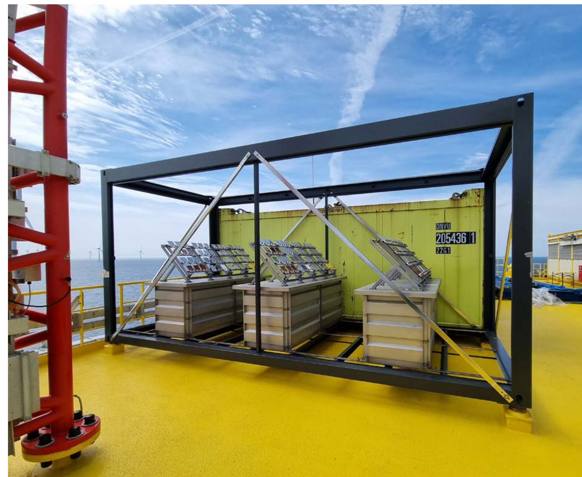
17 different materials and corrosion protection systems are tested for three years, exposed to the elements
