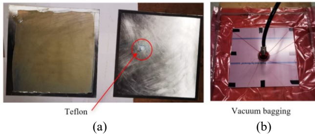
Fig. 9. Fabrication of adhesively bonded aluminum plate: (a) adhesive with artificial disbond using Teflon films and (b) vacuum bagging technique.
