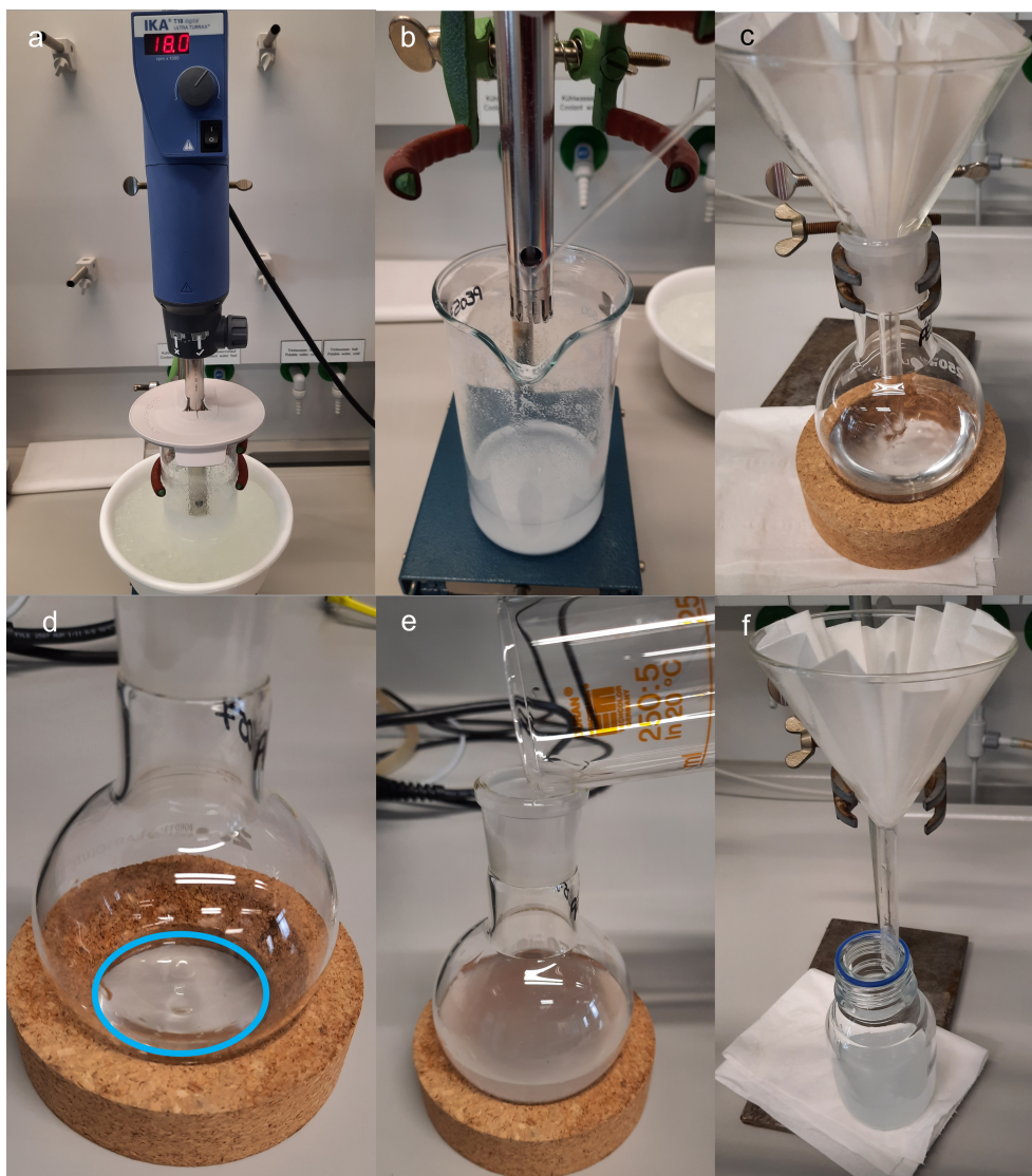
FIGURE 1 Photographs taken of the steps of the nano polypropylene preparation. a) Dispersing the PP in acetone with a Ultra-Turrax disperser ( 18000 \text{ rotations min}^{-1} for 10 min). The acetone is cooled with ice ( 0^\circ\text{C} ) to keep the acetone from evaporating. b) After dispersion, the disperser tool is cleaned with 5 ml acetone. c) Micro and macroscopic residue is separated with a folded filter (pore size of 12 to 15 micrometer). d) An amount of 90 % of the acetone was evaporated; the remaining 15 ml of dispersion in acetone is indicated with the blue circle. e) The addition of 115 ml of water leads to an immediate turbidity of the dispersion. f) After removing the remaining acetone, the dispersion was filtered again to remove possible aggregation products.
