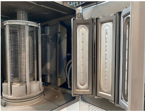
Fig. 1 PVD coating system with substrate electrode [19]
