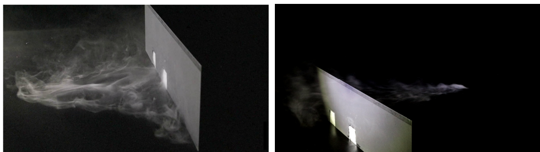
Figure 3. Source locations in the wind tunnel model. Top: schematic view of all source locations, Bottom left: S1 and S2 with haze visualization, Bottom right: S4 with haze visualization.
