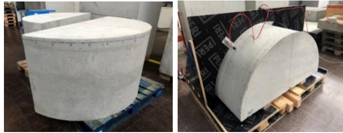
Figure 3: a) Half-cylinder test specimen b) measurement setup
