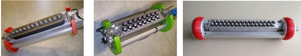
Figure 1: a) Earlier prototype, b) 2 nd generation borehole probe c) New phased array borehole probe
