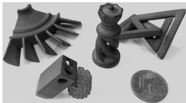
FIGURE 9 SiSiC parts after infiltration showing the capability of the layerwise slurry deposition (LSD-print) process
