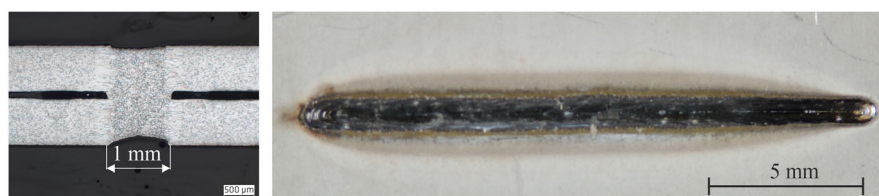
Figure 7. Macrosection (left) and top view (right) of the weld seam for the laser beam-welded shear test specimens.
