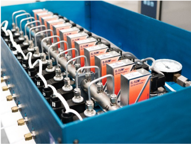
Figure 3. Sampling manifold with valves and MFCs.
