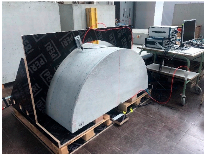
Figure 21. Measurement setup for directivity measurement for third generation probe on concrete half cylindrical specimen.
