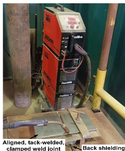
Figure 2. Experimental setup of GMA welding experiments.
