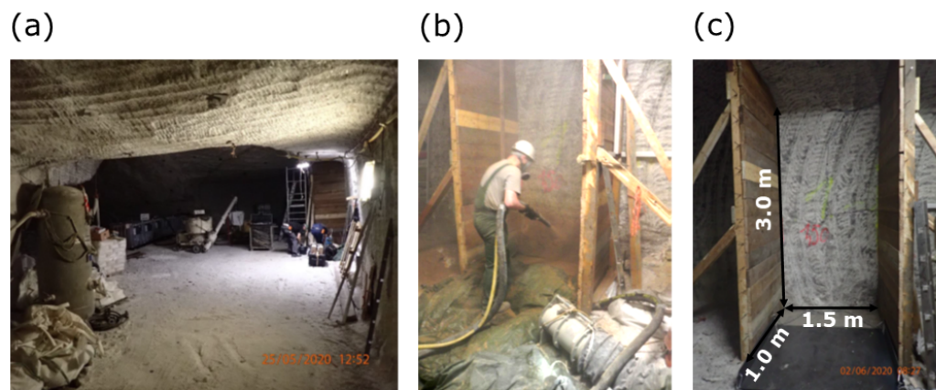
Figure 1. Impressions from shotcrete experiments at Teutschenthal mine: (a) experimental underground site, (b) during shotcrete procedure at a shotcrete box, (c) preparation of a shotcrete box.
