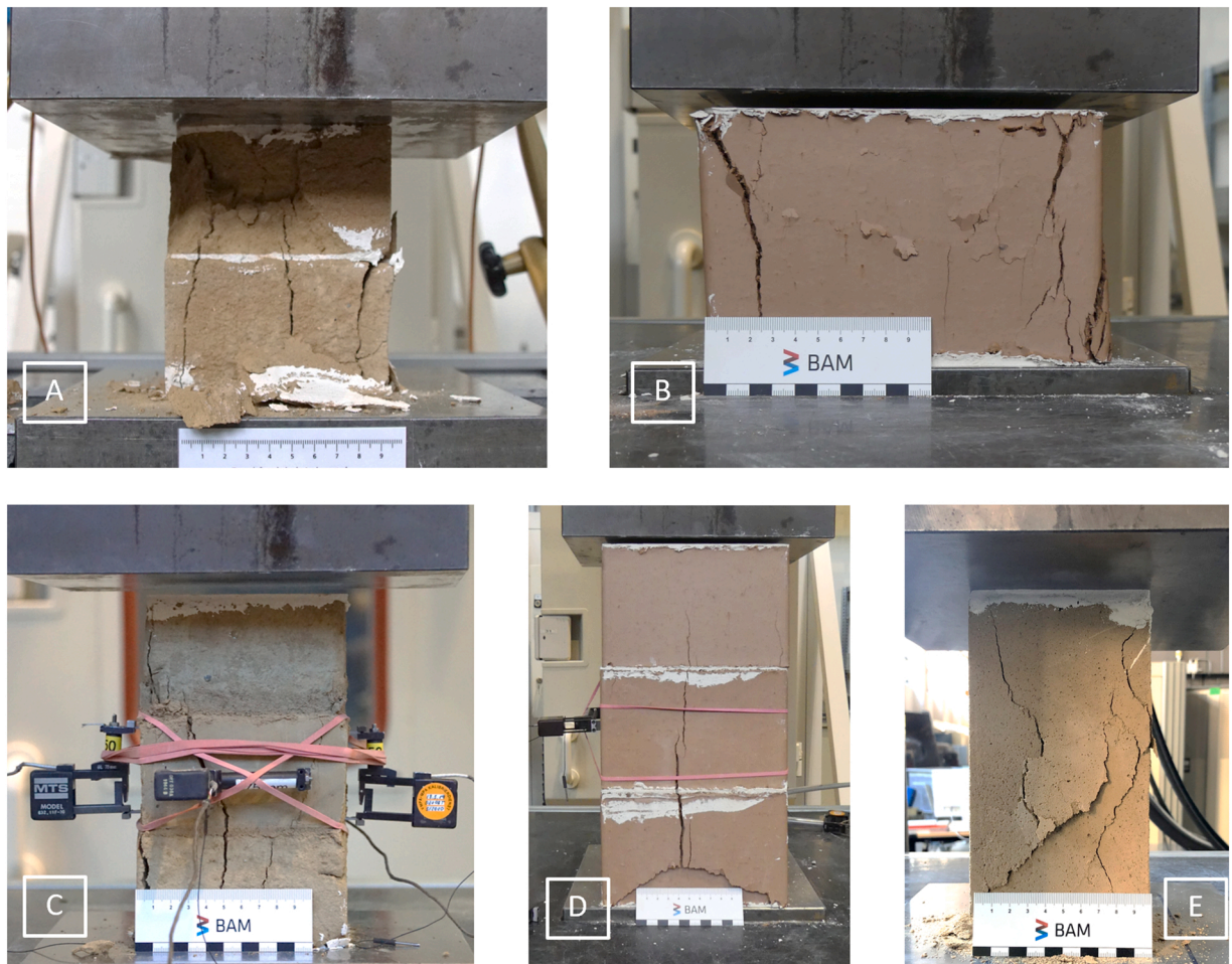
Fig. 4. Cracking patterns of compressive strength samples of NF blocks (A) and 3DF blocks (B) and of NF (C) and 3DF (D) prisms used for deformation measurement as well as cracking patterns of the mortar prisms (E).
